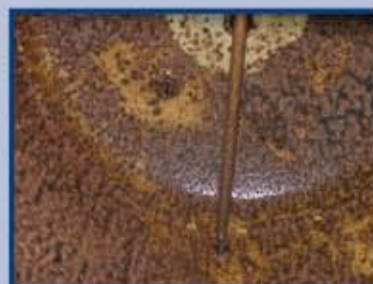
BEFORE A corroded and pitted Domestic Hot Water Storage Tank. If the corrosive action had continued, the tank would soon have required costly replacement.
